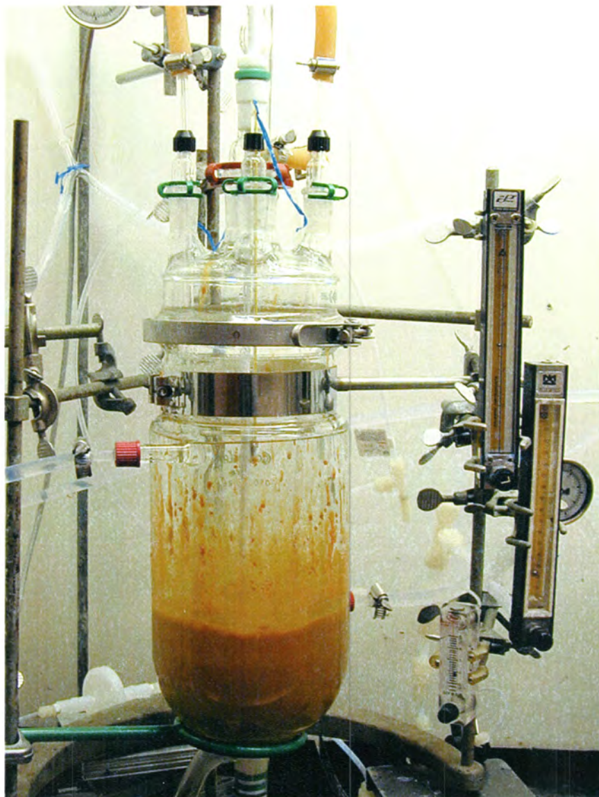
FIGURE A1. PFS synthesis reactor.
